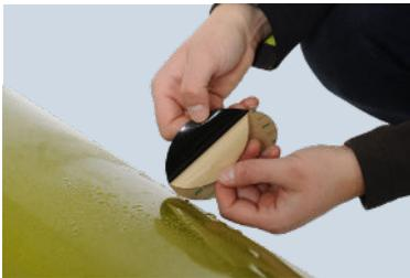
**Repairs in the field:** For quick repair of small holes and tears in the hull, spray deck or seat cushion we recommend the „Anfibio LifePatch“ (self adhesive fabric patch).
