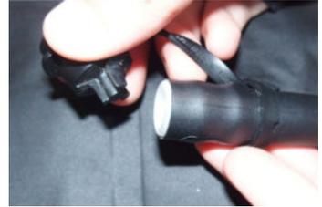
To deflate the seats and backrests press the back of the cap of the non-return valve into the opening, so that the air can escape (see picture on the right). Now push the air out completely.
