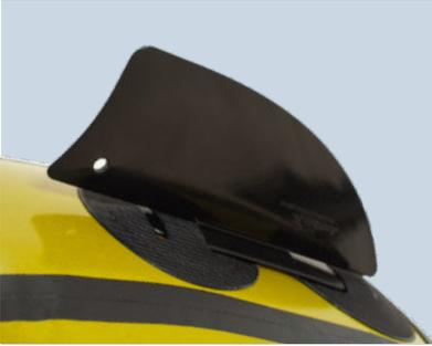
A fin mount is fitted as standard (except Anfibio Nano SL/RTC). It consists of two tabs under the stern of the boat. The optional fin can be easily mounted or dismounted.
