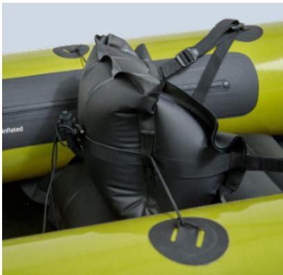
The backrest is to be adjusted adequately to the seat or your body size. To do this, mount the backrest using the pull straps and elastics as shown. The backrest should rest on the rear chamber of the seat.
